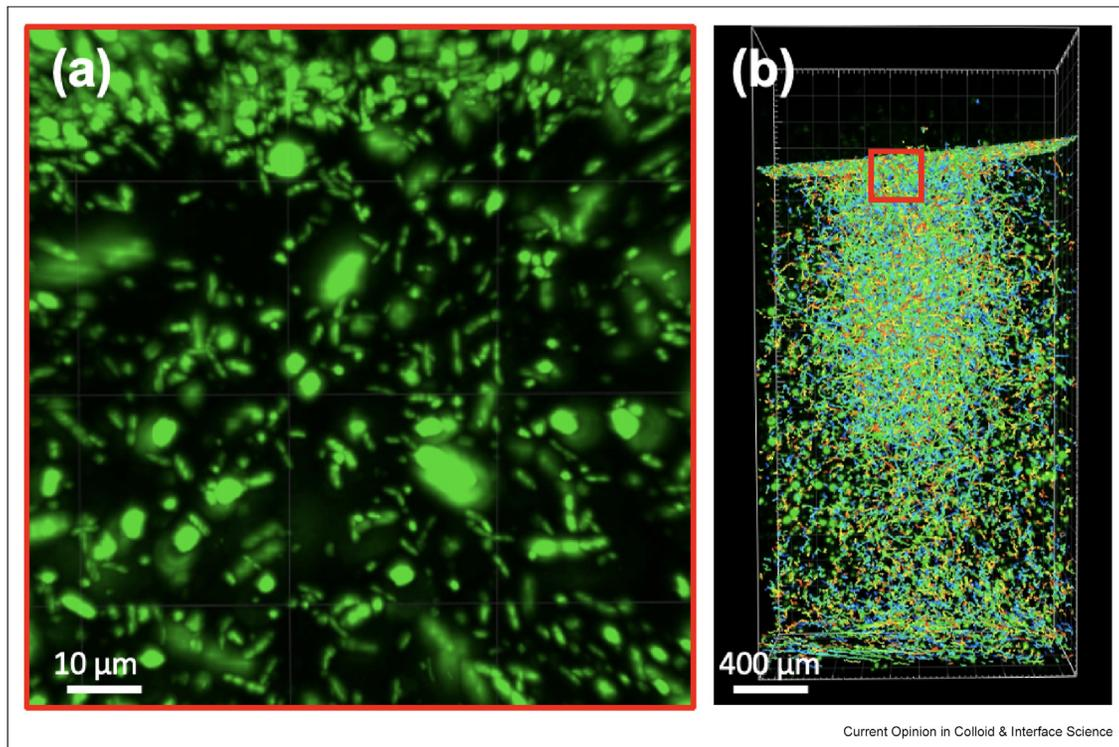
(a) Zoomed-in view of green-labeled yeast (large) and bacteria (smaller, rodlike) within a cellulose pellicle biofilm. (b) Zoomed-out view of sample holding the bacterial culture showing trajectories of all the visible bacteria over the first 10 min of the experiment.
