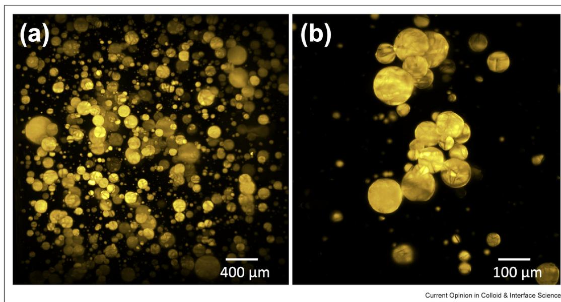
(a) Light sheet fluorescence microscopy (LSFM), 3D reconstruction of droplets of hexadecane-containing paraffin wax crystals imaged within a full emulsion environment. (b) Zoomed-in view of specific droplets with stable and arrested structures. LSFM enables resolution of small details within the droplets, like the arrested neck structure between droplets. Oil is stained here with Nile Red for fluorescence of the liquid phase, while the submicron-thick wax platelet crystals inside appear dark. .
